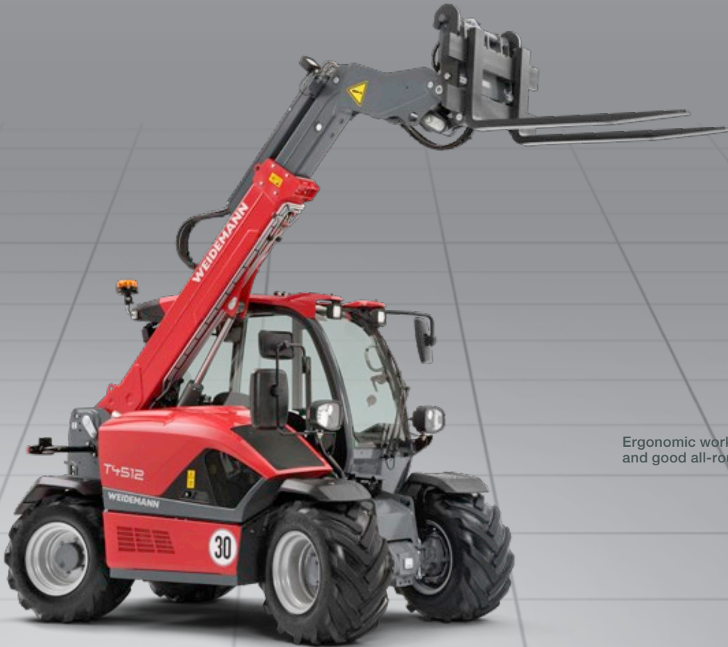
All-wheel steering, low centre of gravity and excellent stability.
