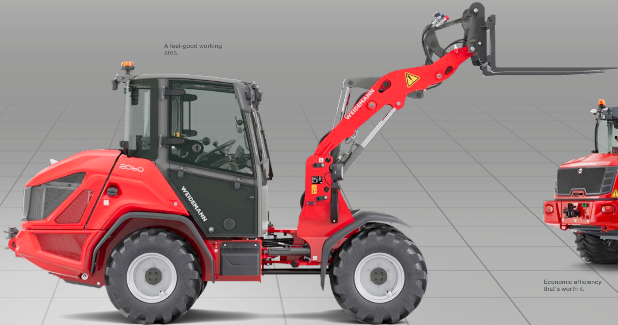
Road capability with articulated pendulum joint.
