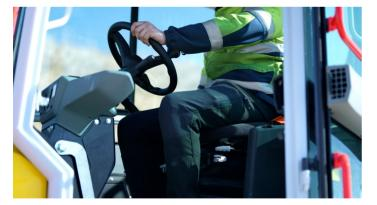
The new rotating seat offers extensive legroom and space for the operator. The operator can move freely and can still turn the seat while sitting, without restrictions.
