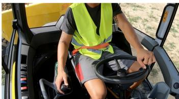
The seat belt monitoring system signals visually and acoustically if an attempt is made to start the machine when the operator is not wearing a seat belt. The additional start release prevents start-up in this case.
