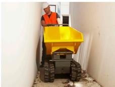
The compact dimensions of the machine make it ideal for manoeuvering and working in confined spaces.
