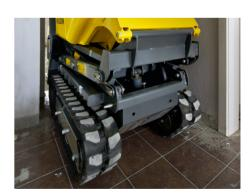
Due to the wide tracks, the machine produces very low ground pressure, which reduces ground disturbance during repair work. This also leads to a more comfortable and smoother driving experience and protects the machine and operator.
