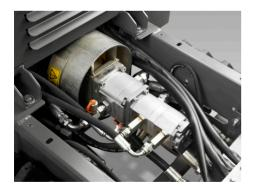
Simply start and off you go: Because of the hydrostatic drive system, no frequent gear changing is needed and the operator can focus on the task. The hydraulic drive system and the working hydraulics can be operated independently of each other.
