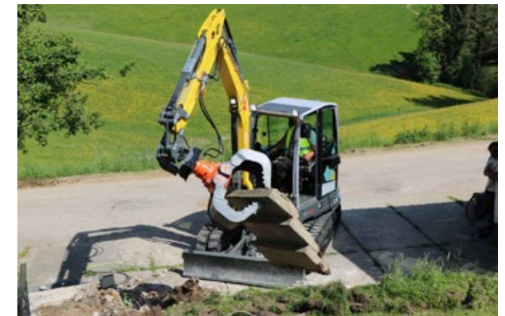
Swivel bucket incl. hydraulic hoses and couplings
