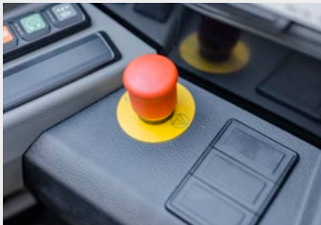
Quick-to-reach emergency button, so that the machine can be immediately brought into a safe state in case of emergency.
