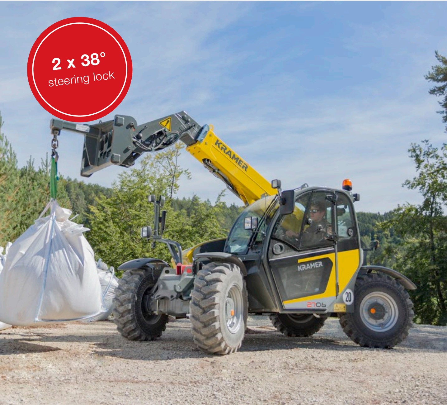
All-wheel steering: particularly manoeuvrable in tight spaces
