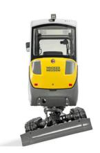
The vertical digging system compensates for slopes of up to 15 degrees, making it possible to vertically excavate on a slope. This is not only ergonomic for the operator, but it also saves time and also means less excavated material.
