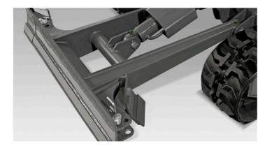
The hydraulically telescoped travel gear with a max. outer width of 1300 mm gives stability. In no time it can be retracted to a width of 990 mm. With the foldable dozer blade extension, this makes individual adjustment to the job site conditions possible. Meanwhile, the extension elements are always connected to the machine and therefore do not get lost.
