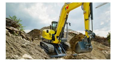
The powerful drive system combines with a load-sensing hydraulic system (LUDV) to deliver quick working cycles, greater application flexibility, and easier control for comfortable and fatigue-free operation of the excavator. No matter what the load to be moved, the control movements on the joystick stay the same. Along with increased operating comfort, this results in a performance plus, while simultaneously reducing fuel consumption.
