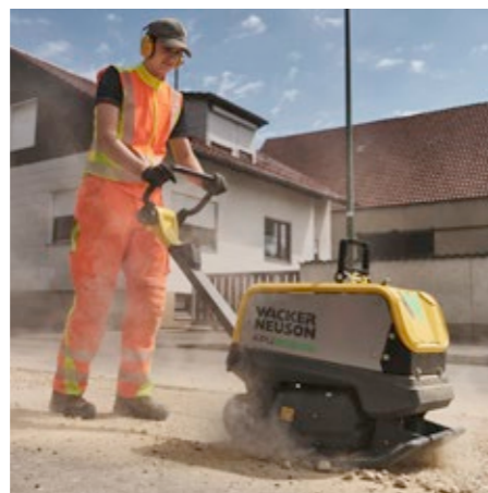
With one battery charge, the APU3050e compacts up to 333 m 2 soil*.
