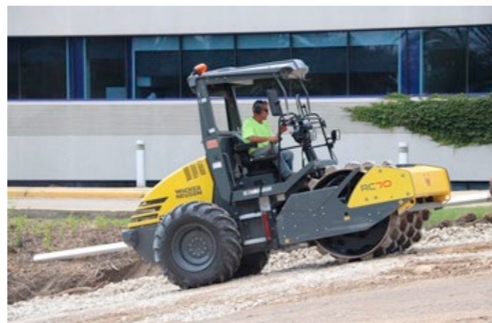
Traction control ensures that the wheels do not spin even on uneven terrain.
