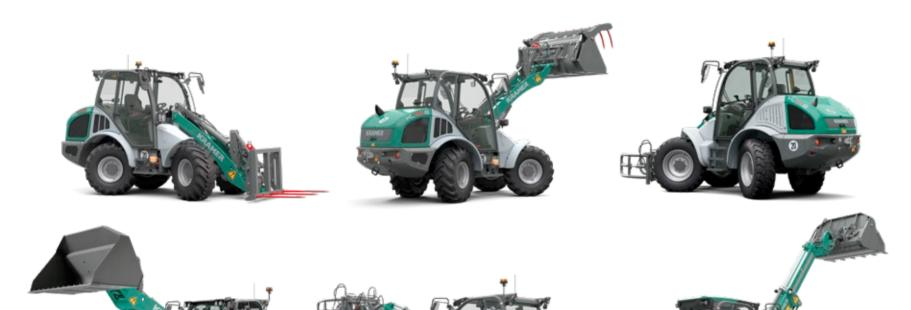
**OPERATING AND PERFORMANCE DATA** KL36.8 KL36.8L KL38.8 KL38.8L Engine output standard [kW] 55.4 55.4 55.4 55.4 Engine output option [kW] -\_ \_ Bucket capacity [m3] 0.85 0.75 0.95 0.85 3,650 3,000 3,890 3,240 Bucket tipping load [kg] Stacking payload S=1.25 [kg] 2,150 1,850 2,300 1,950 Operating weight [kg]\* 4,600-5,200 4,600-5,200 5,000-5,600 5,000-5,600
