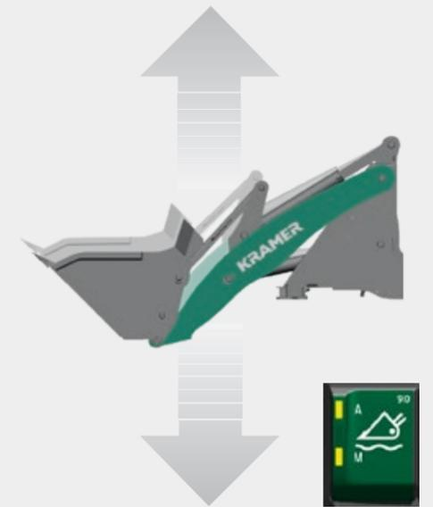
**The load stabiliser dampens oscillations** of the load stabilizer, providing for improved ride comfort and increased driving safety.
