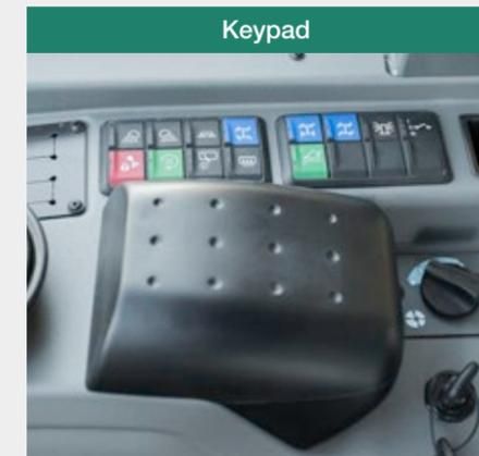
The respective functional group is very quick and easy to identify due to the colour-coded switches. Red = safety, green = hydraulics, blue = travel and grey = electrical system. This ensures the operator a convenient and safe operation without the risk of being confused. The result is increased working efficiency.
