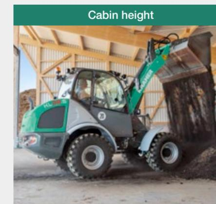
The compact and low design of the wheel loaders of less than 2.50 m allows for the ideal application of the machines in confined farm yards and stables. The machines have the best arrangements for low clearance heights thanks to their design.
