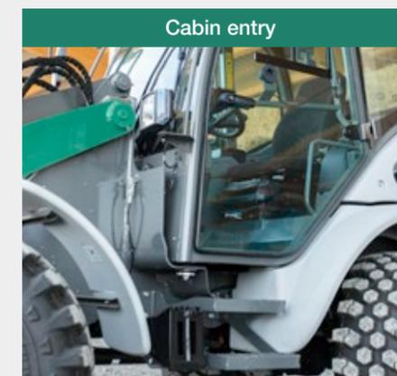
The cabin can be accessed through the large entry area. A two-stage entry is optionally available to give the operator an even more comfortable entry.\* In addition, the handles are in an ergonomically favourable position.
