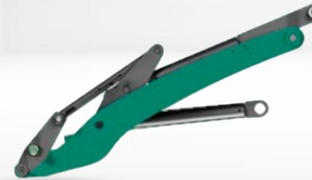
The parallel-guided loader unit ensures constant lift capacity and a safe operation in materials handling. Due to the 50° high tilt back angle and the tilt-out angle of 45°, the wheel loader does not lose any material in bucket application, even when it is very full, allowing for a complete emptying of the bucket.
