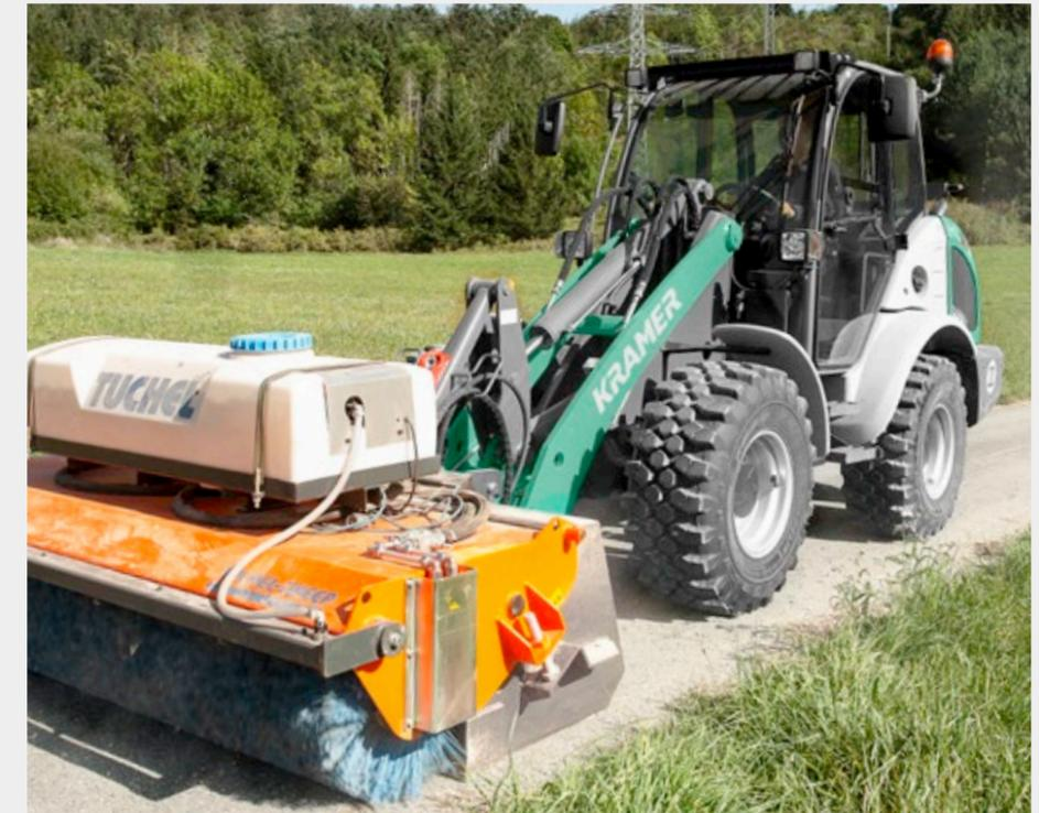
**CSD - constant travel speed:** supports compliance with the set speed, especially when running attachments where a consistent speed is required for the correct execution of the work process, such as: snowblower protection, rotary sweeper or mulcher.
