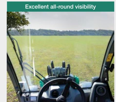
The central seat position in combination with the large glass windows offer a 360° all-round visibility. The particularly clearly-arranged design and the seat position of the operator avoid "blind spots". You can even see everything to the rear. The elevated front window allows for a perfect view of the attachment, even when the loader unit is raised.
