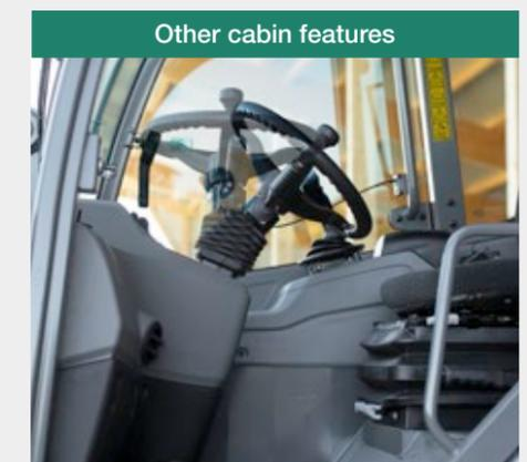
The extensive standard equipment includes, among other things, the tilt-adjustable steering column, which is individually adjustable. In addition, the rear-view mirror and the four work lights offer an optimal line-of-sight. The vehicle can optionally be equipped with an air-sprung driver's seat with lumbar support and a heated seat.
