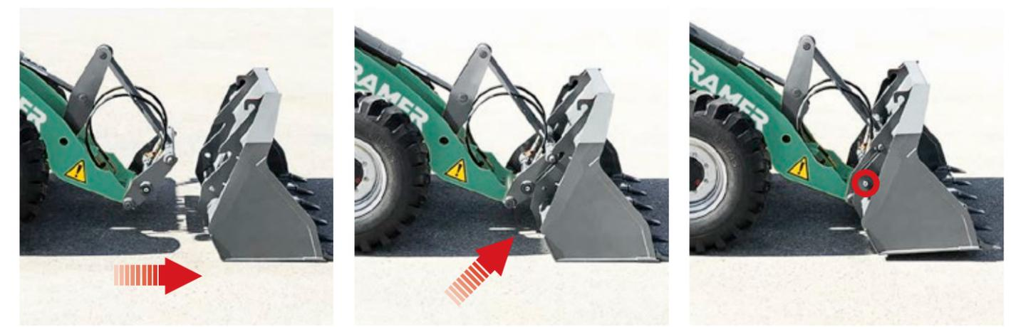
**Hydraulic quick-change system - The Kramer quickhitch system:** approach the attachment, pick up the attachment hydraulically from the operator's seat and lock it using the touch slide on the joystick. The lock cylinder is located above of the pivot point of the quickhitch plate and is thus not in the contamination area.
