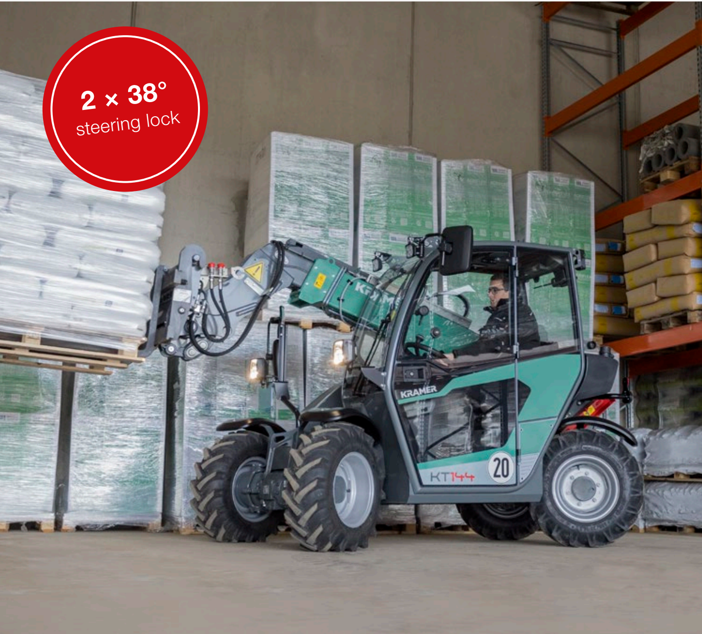
All-wheel steering: particularly manoeuvrable in tight spaces
