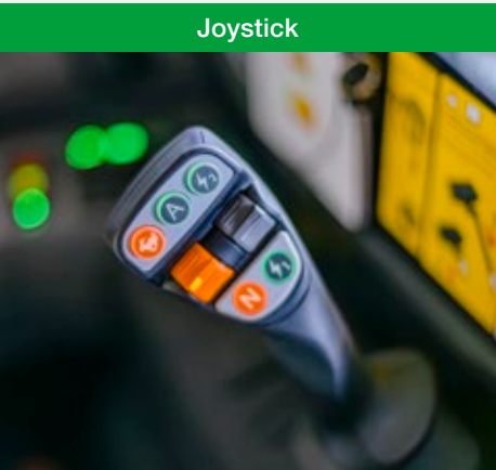
The operator has everything under control with the multifunctional joystick. Alongside the main functions of lifting and lowering, as well as feeding and tipping out, all of the important functions are included on the joystick, i.e. selection of travel direction. Additionally, the operating elements of the joystick are backlit in the dark, which guarantees safe operation of the machine, even in the dark.
