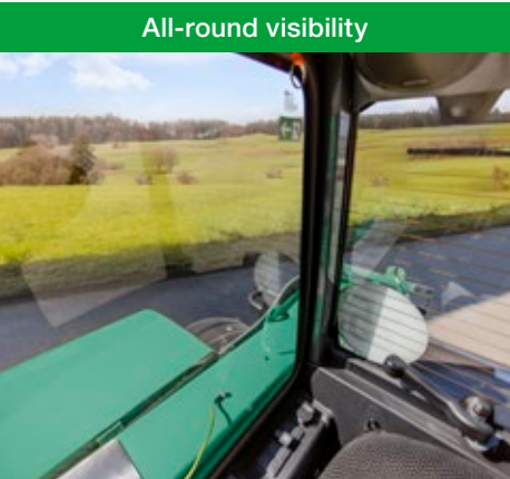
Narrow cabin struts and panoramic glazing enable an excellent view on all sides. The panoramic front windscreen contributes to a good overview and improves the operator comfort. The flat battery cover ensures an optimal view to the right side, on the right rear wheel and the wing.
