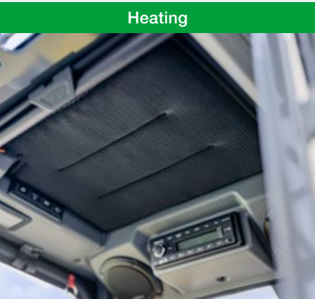
The machine is equipped as standard with a cabin windscreen heating. So that the highest possible level of energy efficiency is achieved for the overall heating system, the cabin can be equipped with auxiliary panel heating for normal air heating. This is in the cabin roof and provides targeted heat. The normal air heating can also be used as standard heating during the charging procedure.
