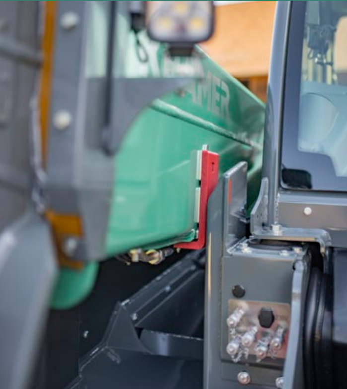
Lateral guidance of the loader unit
