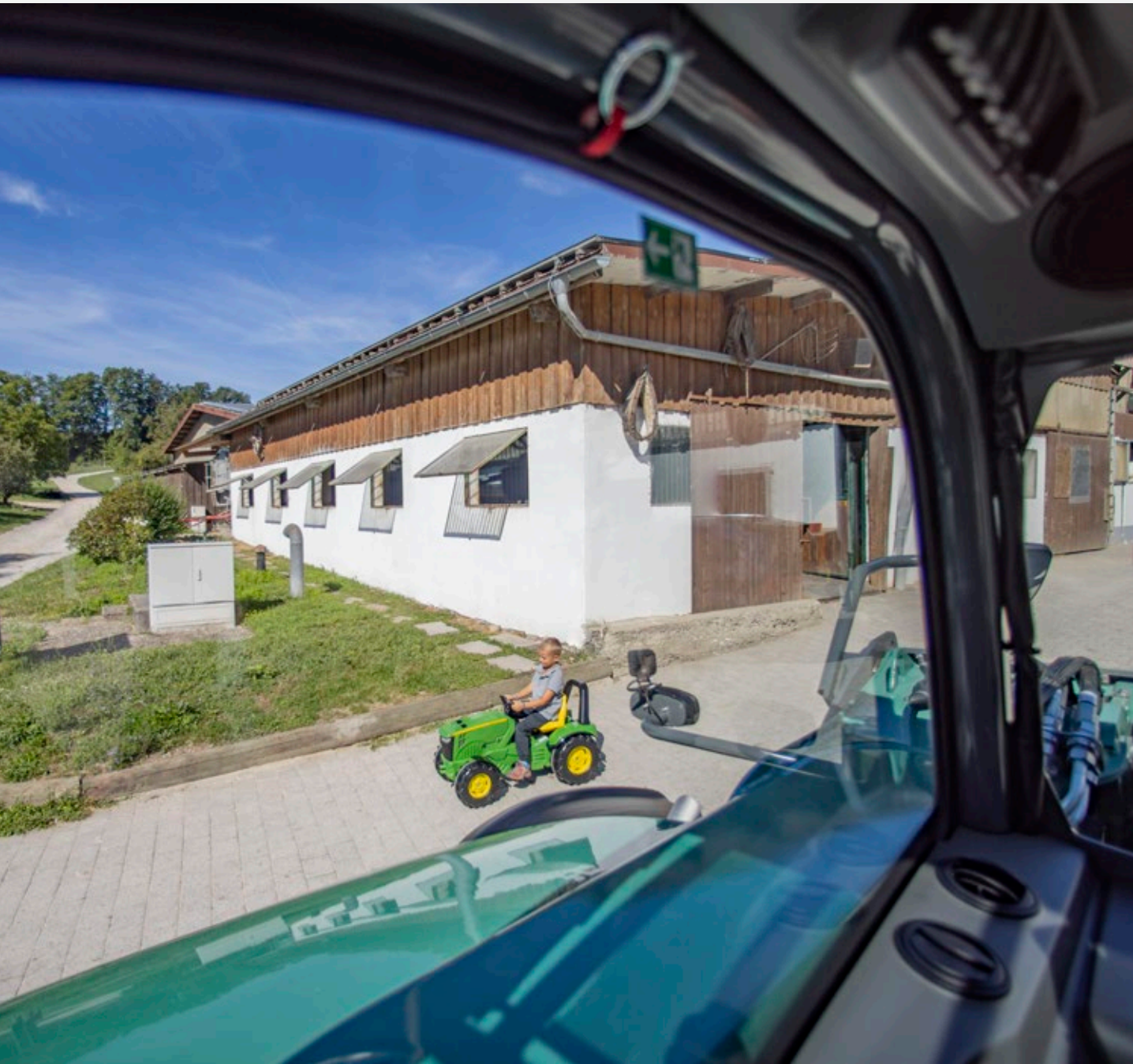
Flat engine cover ensures optimum visibility to the right.
