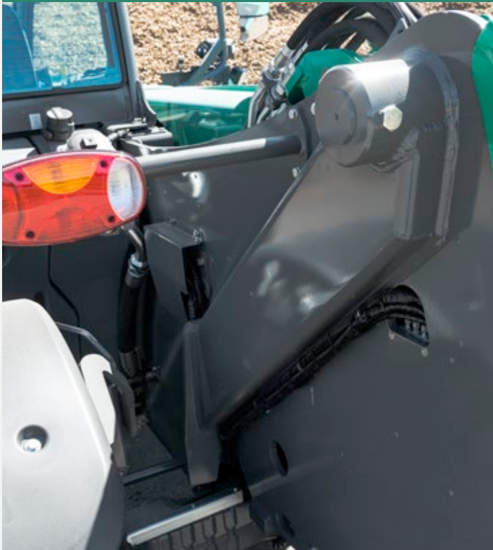
Frame reinforcement at the main bearing
