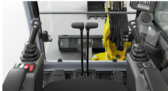
The intuitive operating concept enables simple and comprehensive control of the excavator. The machine is operated using a joystick, jog dial and keypad. This makes accessing attachment and oil level settings for the additional control circuits quick and easy.
