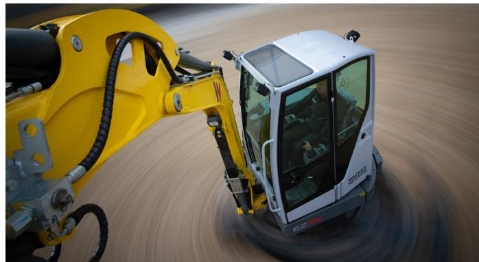
The large, fully glazed and tiltable cabin with roof window offers the operator an optimal 360° visibility of his work area. This gives the operator a good view of his working area, colleagues and any dangers. Meanwhile, available despite this. It can be easily disassembled for service and repair work. All hydraulic functions of the excavator meanwhile remain available.
