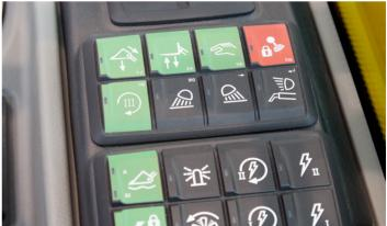
Efficiency during work with the machine is increased due to simplified operation. The colour-coded switches increase safety by reducing the danger of confusing the switches. This way, even new operators quickly find their way around the machines.
