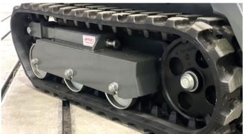
The suspension-mounted rollers provide for a smooth and safer operating experience. Due to the suspended support, the rollers adapt to the terrain and compensate for obstacles or unevenness, such as stones. As a result, the operator benefits from optimal driving comfort, even off-road.
