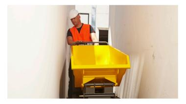
Simply start and off you go: Because of the hydrostatic drive system, no frequent gear changing is needed and the operator can focus on the task. The hydraulic drive system and the working hydraulics can be operated independently of each other.
