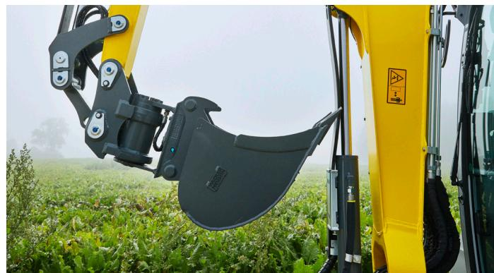
The cylinders and the cylinder rods are protected from damage thanks to the plastic rails, which lengthens their service life and saves costs. Due to their flexible material, they return to their original shape after an impact. Their appearance and characteristics are completely retained.
