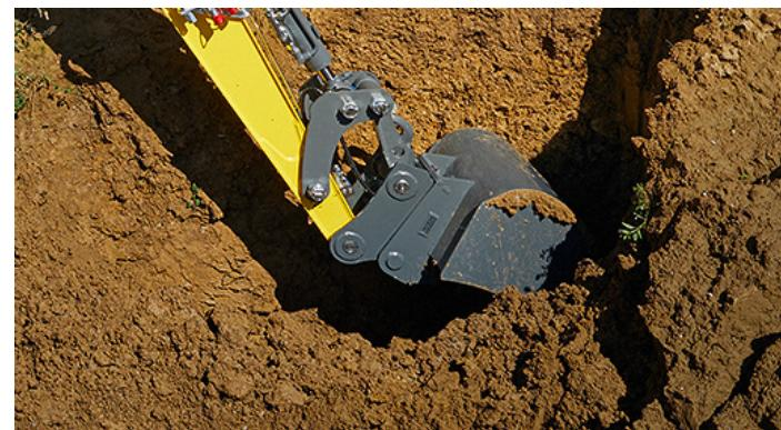
With 3-point kinematics, the conventional bucket linkage has been taken to a new level. This "3-bolt" design extends the bucket's angle of rotation to 200 degrees - 10% more than conventional bucket linkage. This increases the vertical dig depth as well as the digging forces. This eliminates the need to reposition the excavator as often, significantly increasing efficiency.
