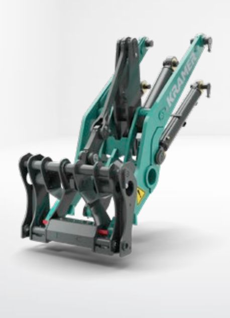
Standard loader unit (PZ-kinematics) with Kramer quickhitch plate
