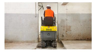
The Roll-Over-Protection-Structure (ROPS) serves as protection against rollover. For low passes or for easier transport of the machine, it is simply folded down without causing rear overhang.
