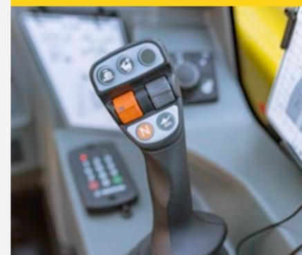
You have the whole machine under control with the ergonomic joystick. With up to 17 functions on the joystick, you have the most important machine functions at your fingertips in one hand.
