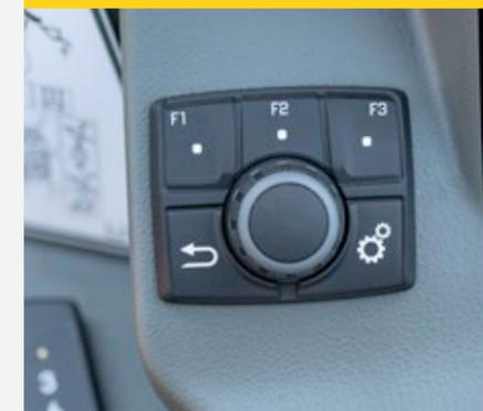
The cabin is equipped with a so-called jog dial. This makes it possible to easily adjust all important machine settings, such as the oil volume of all control circuits. The most important operating data can be shown with the rotary and push wheel and adjusted entirely to the operator's needs.
