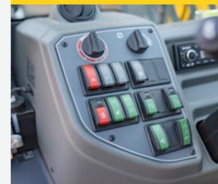
All switches and buttons of the machine are colour-coded so that the operator can find the desired function faster. The buttons with a safety function are red, those for the hydraulics are green, for the electrical system grey and for the drive system blue. All controls are backlit, so you are always able to use the right switch even in the dark.
