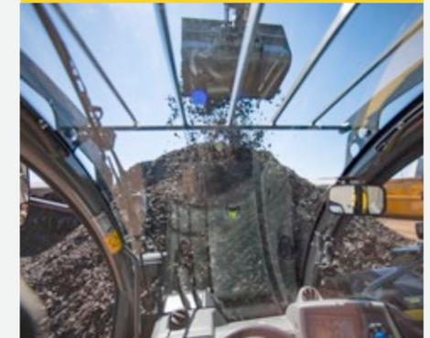
Everything always in view. All Kramer telehandlers have a continuous front window without disturbing cross braces. The window has been pulled up and down as far as possible so that the operator can see the lock pins immediately when changing attachments and still has the attachment in the line-of-sight at maximum stacking height.
