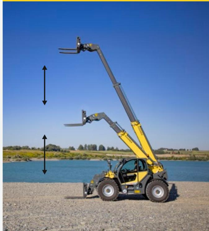
When lifting and lowering the loader unit, the attachment is moved up and down in a vertical line, i.e. the telescopic arm automatically moves in and out and the load is moved up or down in a straight line. Thus, the cargo always remains in the safe range and stacking work at high altitudes is simplified.
