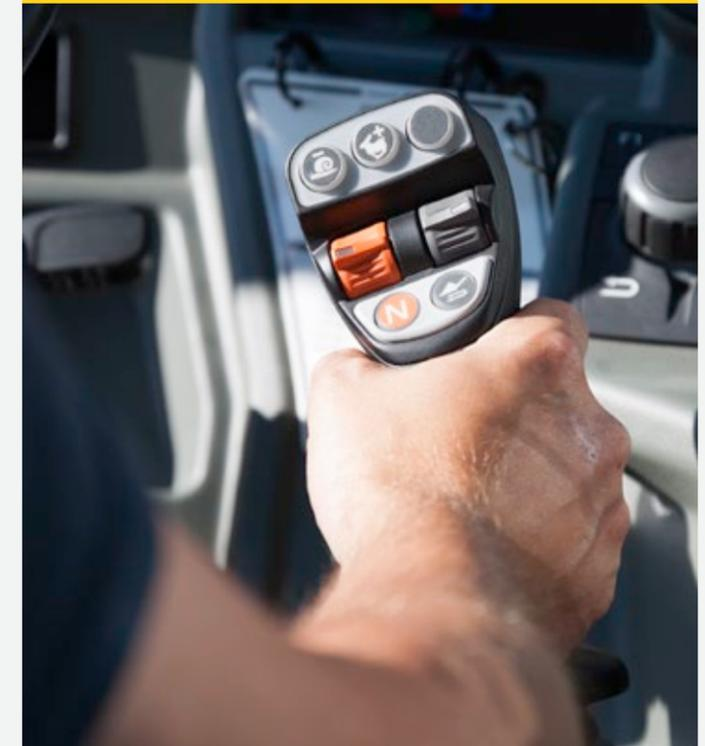
You have the whole machine under control with the ergonomic joystick. With up to 17 functions, the most important tasks can be done without letting go of the joystick or changing your grip. For models from the 3007 through to the 3610, the joystick is attached to the cab console. For the models of performance class 4507 through to 5509, the joystick is affixed directly to the operator's seat.
