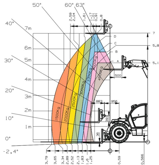
**5509** Load-bearing capacity diagram (with LSP 600 mm) with hydraulic level compensation and oscillating axle interlock
