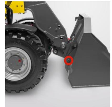
**Hydraulic quick-change system (optional) - The Kramer quickhitch system:** Approach the attachment, pick up the attachment hydraulically from the operator's seat and lock it using the touch slide on the joystick. The locking cylinder is located outside of the pivot point of the quickhitch plate and is therefore not in the contamination area.
