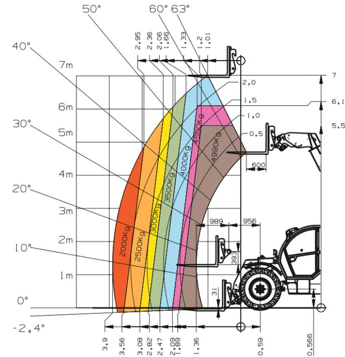
**4507** Load-bearing capacity diagram (with LSP 500 mm)
