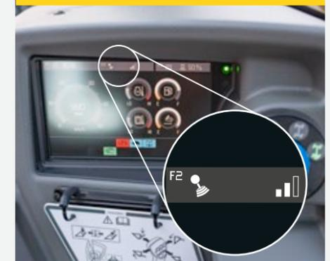
The display and the jog dial can be used to adjust the speed of the work hydraulics for lifting and lowering the lifting arm as well as tilting in and out the attachments in three stages. This allows the operator to always choose the right balance between speed and precision.
