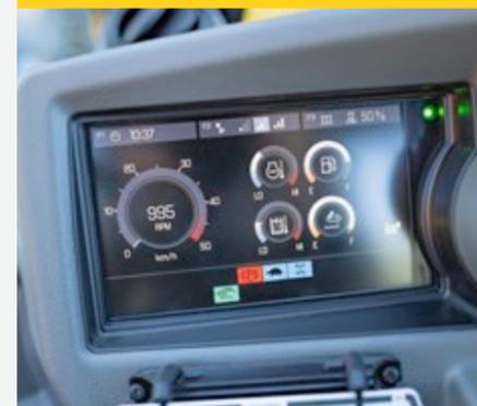
The telehandler has a modern control panel with large 7-inch LCD display. The setup of the display is simple and intuitive. All important vehicle data and functions are shown in the main menu. The brightness can be regulated and customised to your needs. The optional rear-view camera provides an improved view to the rear.
