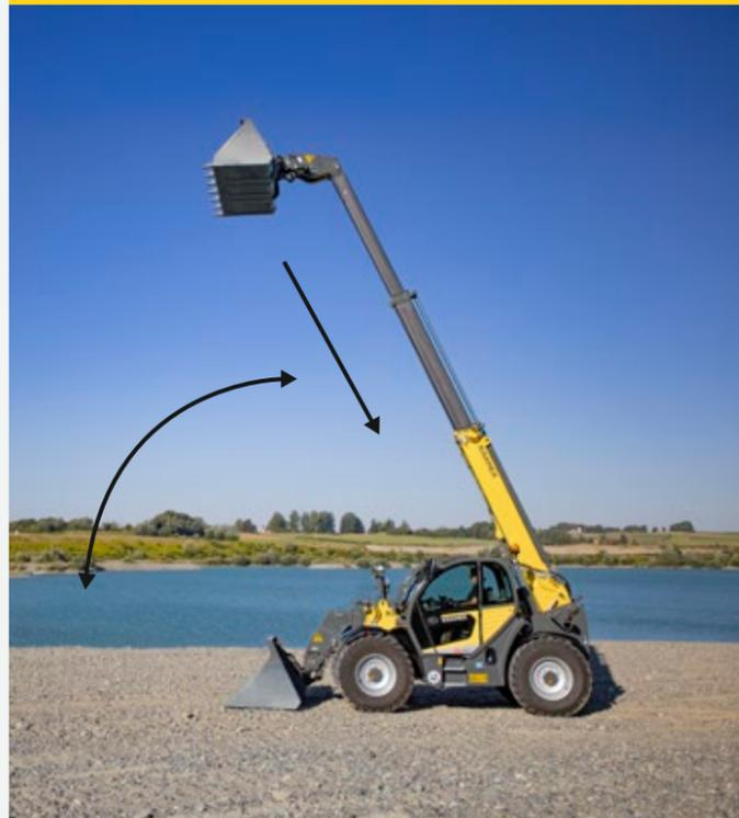
When lowering the loader unit, the telescopic arm is automatically retracted. This keeps the load as close to the vehicle as possible and it does not create critical situations, even with maximum payloads. The bucket mode is ideal for loading bulk materials.
