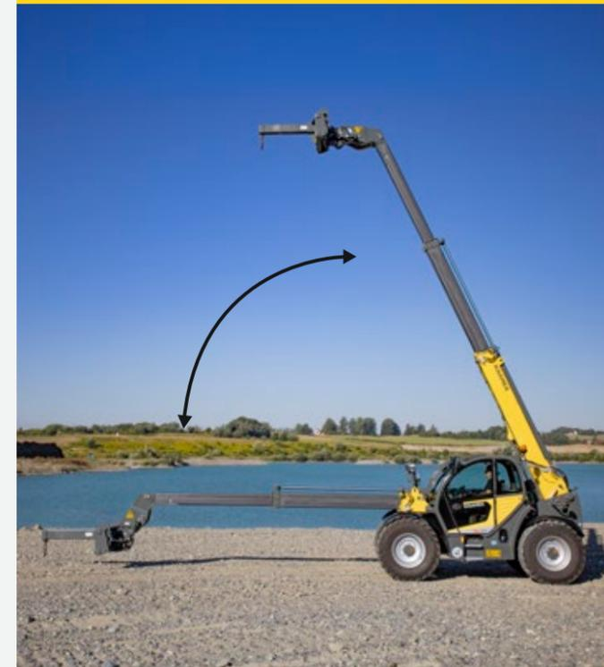
In manual mode, the machine does not perform any automatic movements of the loader unit. The overload protection is of course still active and stops the loader unit as soon as the overload limit is reached. At this point, only retracting, lifting the loader unit and dumping out the attachment are possible.
