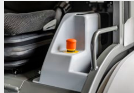
Quickly accessible emergency switch, so that the machine can be immediately put into a safe status in an emergency.
