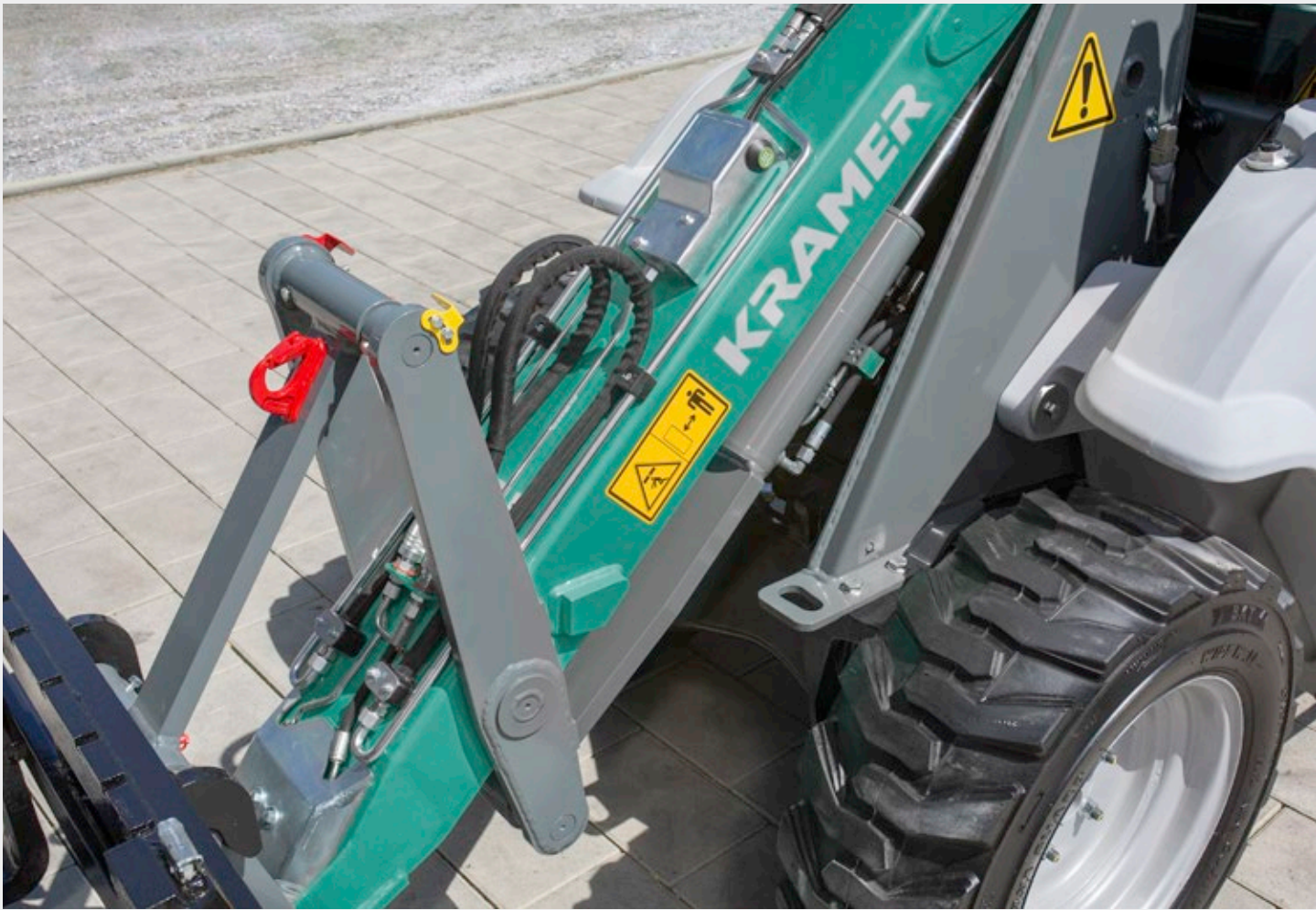
Sturdy loading system with Z-kinematics, visual position indicator and optional load hook.
